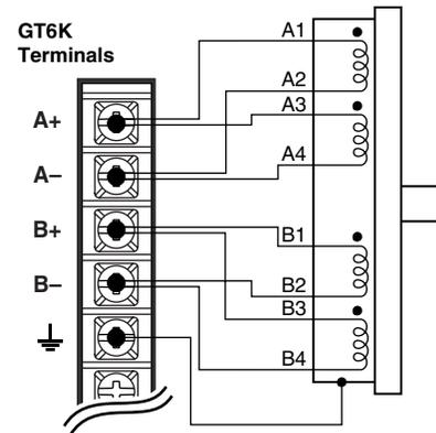
*Non-Compumotor Motor Connections*
