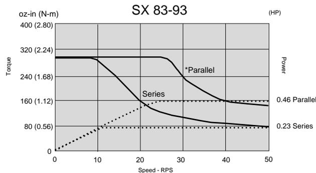
\*Parallel connected motors are limited to 50% duty cycle when operated above 5 rps. For greater than 50% duty cycle above 5 rps, you must connect the motor in series. Fan cooling the motor will increase duty cycles above 5 rps.
