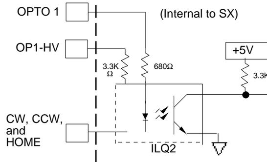
Note: OPTO1 is for use with (5-12VDC) power supplies and OP1-HV is for use with (12-24VDC) power supplies. They should not be used together.
