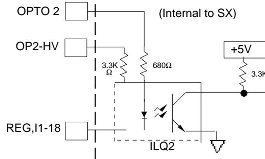
Note: OPTO2 is for use with (5-12VDC) power supplies and OP2-HV is for use with (12-24VDC) power supplies. They should not be used together.
