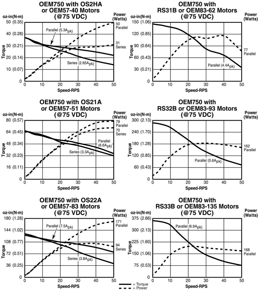
Note 1: Parallel connected motors are limited to 50% duty cycle when operated above 5 rps. For greater than 50% duty cycle above 5 rps, you must connect the motor in series. Fan cooling the motor will increase duty cycles above 5 rps.
