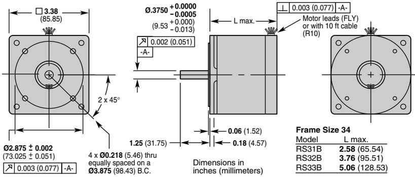
Size 34 Frame, RS Series Motors, Regular Construction
