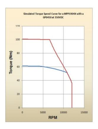
Notice that there is roughly a 17% difference between the peak and continuous output power. The ability for the Parker motor to accomplish this is through our proprietary dual-cooling configuration
