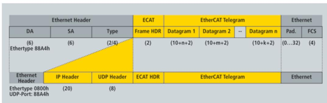
**Figure 3:** EtherCAT: Standard Frames according to IEEE 802.3
