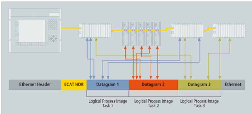
**Figure 2:** Process data is inserted in telegrams
