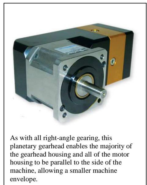
300 rpm. Driving this load with a servomotor alone (assuming industry-standard performance characteristics) necessitates a 142-mm frame size and a drive supplying 30 A continuous. Such a system costs about \$6,000. In contrast, including a gearhead cuts motor and gearhead frame size to 90 mm — and the resulting mechanical advantage permits a smaller drive as well. Such a system costs about \$3,300.
