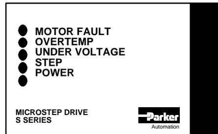
The **MOTOR FAULT** LED is **red** and turns on when the amplifier is disabled. The Fault LED will be activated when any of the following conditions occur:
