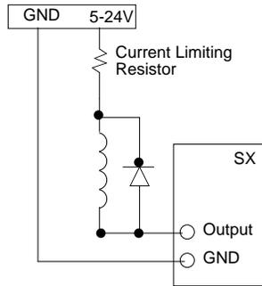
If an inductive load is used, you **must** put a diode across the load, with the anode connected to the SX output (see previous figure). These outputs can sink up to 35mA.
