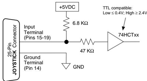
This input circuit applies to Axes Select, Velocity Select, Joystick Release, Joystick Trigger, & Joystick Auxiliary.
