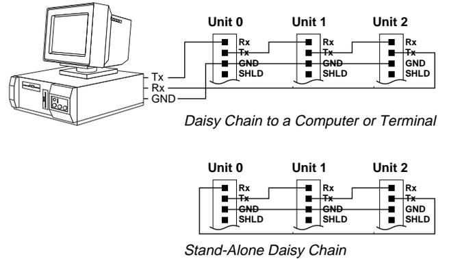
\* Be sure to set unique device addresses for each unit. To set the address, use the DIP switch (see page 4), or use the ADDR command (see 6000 Series Software Reference).
