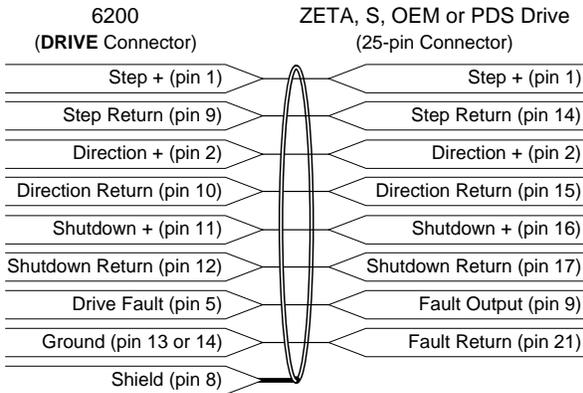
Use the [Z1-010432-10](#) 10-foot cable for plug compatibility with ZETA, S, OEM, and PDS.
