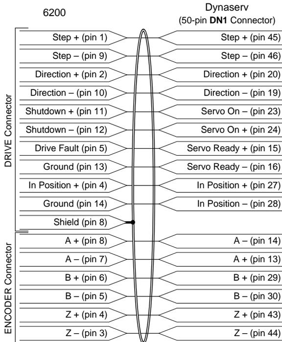
Order the [Z1-012985-10](#) 10-foot cable for easy plug compatibility with the Dynaserv.
