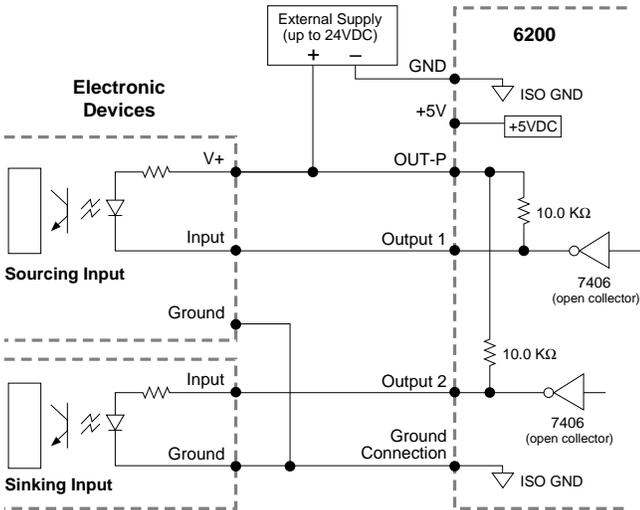
Combinations of sourcing and sinking inputs can be accommodated at the same voltage level. Be aware of the input impedance of the sourcing input module, and make sure that there is enough current flowing through the input module while in parallel with the OUT-P pull-up resistor.
