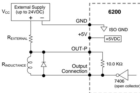
Use an external diode when driving inductive loads. Connect the diode in parallel to the inductive load, attaching the anode to the 6200 output and the cathode to the supply voltage of the inductive load, via an external resistor. To size the external resistor, use this formula:
