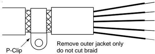
Figure 2. P-Clip Installation
