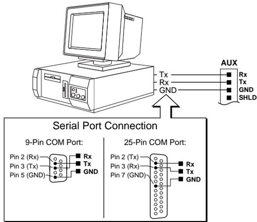
**NOTE:** Maximum RS-232C cable length is 50 feet (15.25 meters)
