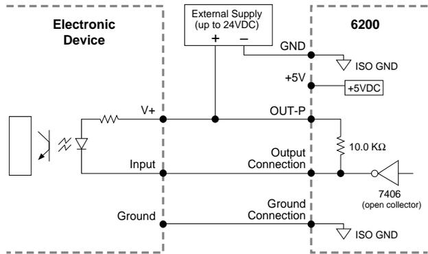
**Connection to a Combination of Sinking & Sourcing Inputs**
