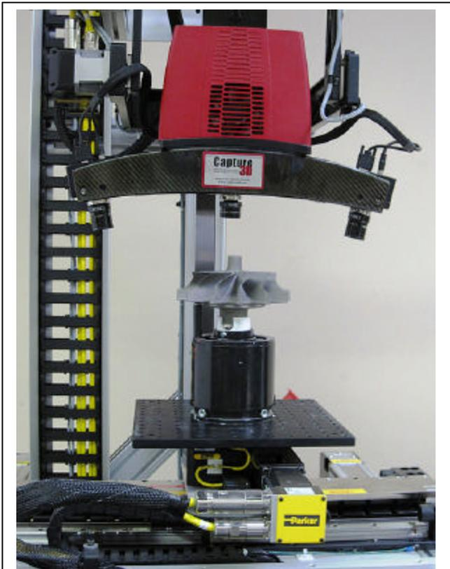
Ethernet Powerlink's ability to precisely deliver motion commands enables this 3D scanner to gather data on an impeller.
