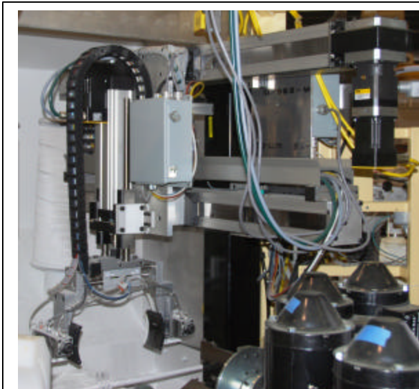
Uncoated generator parts are gripped, picked up and rotated, then transferred into the powder coat process with custom Parker mechanics and controls.
