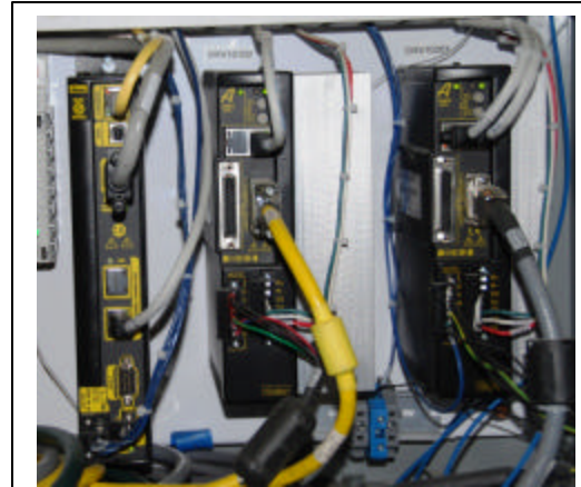
Closeup view of Parker's ETHERNET Powerlink enabled 9040 Controller and Aries drives. The controller and drive are set up and programmed from the same software package, lowering startup and installation costs.
